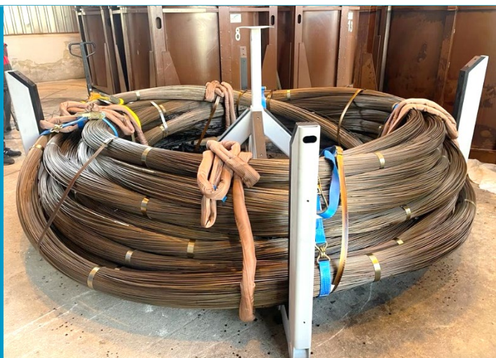
Completed tendon for delivery to Ukrainian NPP, 2024
